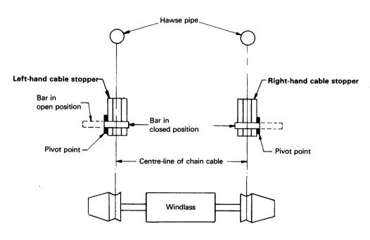
NOTE — Figure 1 is included for information only. It does not imply that the bar is the only possible means of blocking. Other means (for example those in screw-type stoppers) can be used.
